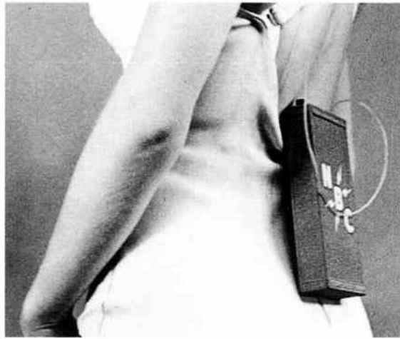
Photo shows "the radio ear" strapped to the back of a performer. The device allowed the director in the control room to talk to stage managers, actors and musicians.
