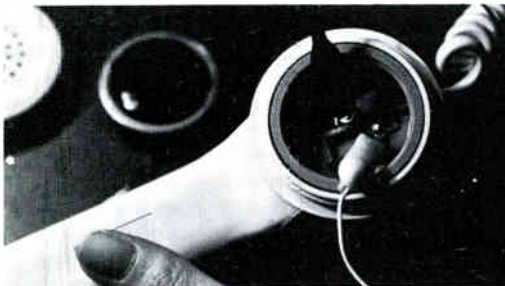
To prevent the clips from touching each other, rubber or plastic sheaths are recommended. This receiver is now ready for "phone-feeding."
