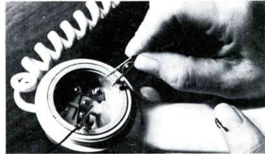
The second clip is attached in a similar manner. It doesn't matter which clip goes to which tongue, as long as the clips don't touch each other.
