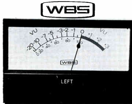
Figure 14.3. 0 VU Meter Reading. A "0 VU" reading on the standard VU (volume unit) meter. Note that the scale above the line is calibrated in dB (decibels) relative to "0" or "reference level," and the scale below the line is calibrated in percentage of modulation for broadcast transmitters. "0 VU" equals 100% modulation. (Photo by Skip Pizzi.)
