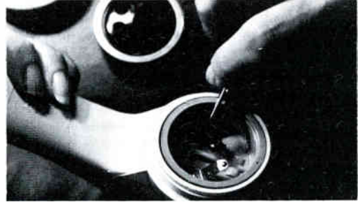
Attaching the first alligator clip to one of the receiver's "tongues."
