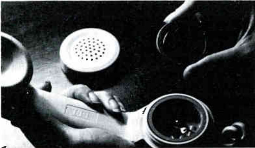
Removing the microphone by lifting it out of the receiver.
