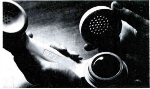
Removing the mouthpiece cover, revealing the carbon microphone.
