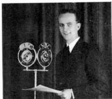
Double microphone stand of NBC employed until 1929.
