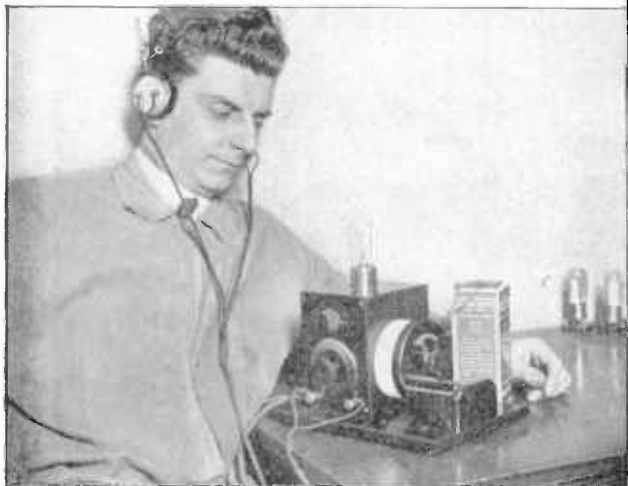
MINIATURE TRANSMITTING AND RECEIVING SET FITTED INTO A CAMERA CASE. MADE BY STERLING G. SEARS (ABOVE), AND WILLIAM A. BRUNO WITH EFFICIENT RECEIVER USING ONE DRY CELL INSTEAD OF STORAGE BATTERY
