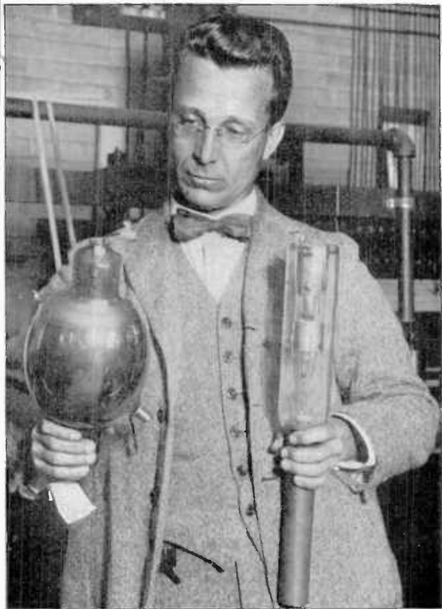
PROF. J. H. MORECROFT OF COLUMBIA UNIVERSITY COM- PARING AMERICAN 20-KILOWATT WATER-COOLED TUBE (HELD IN LEFT HAND) WITH BRITISH AIR-COOLED TUBE OF ONE-HALF KILOWATT
