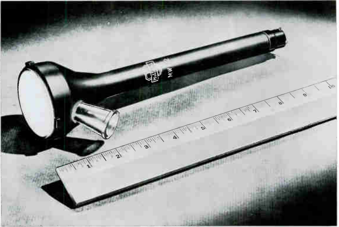
The 2 1/2" tube used in projection sets in the early-1950s
