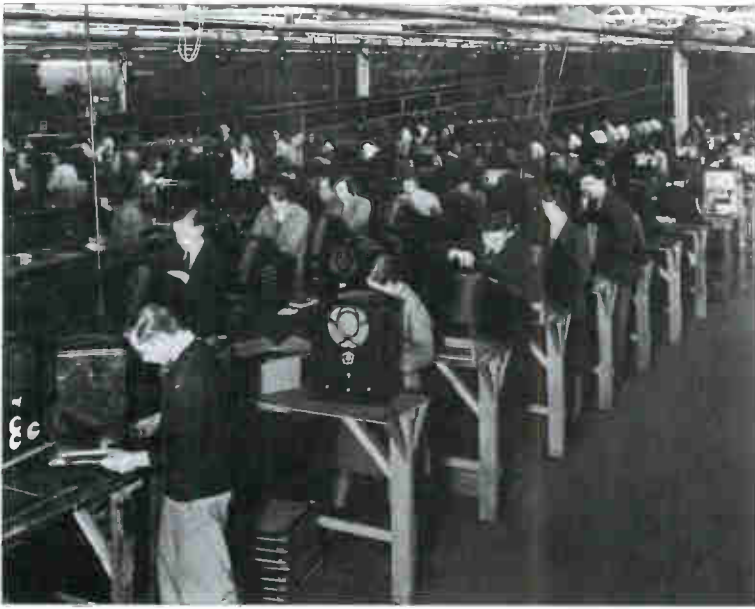
Final testing of K-B Model 279. 1931. Untypically for a radio factory of the period, men and women are working on the same task
