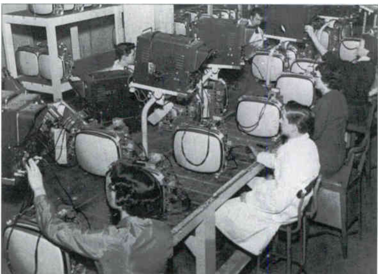
A 'hot track' enables receivers to remain powered as they move along to successive alignment stations, c. 1959
