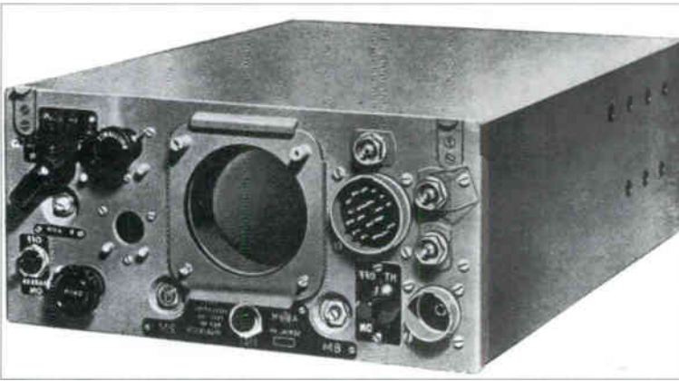
The AI Mk VIII, an airborne interception radar developed and built by Ekco
