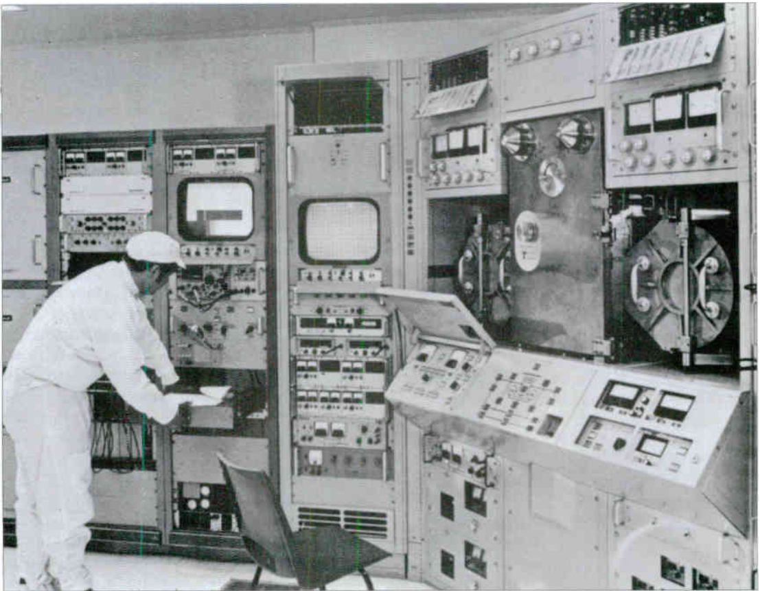
The electron-beam recording plant built at Basildon by the EVR Partnership to make films for the system
