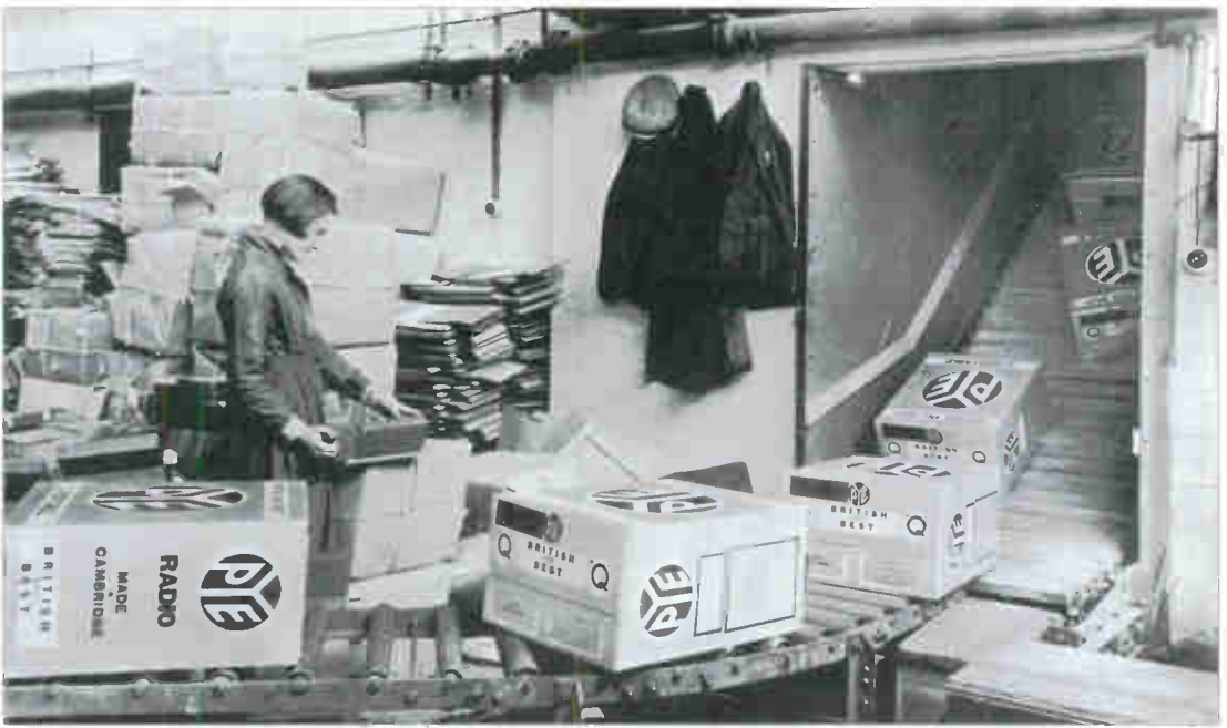
Cartoned receivers being taken up by the elevator...
