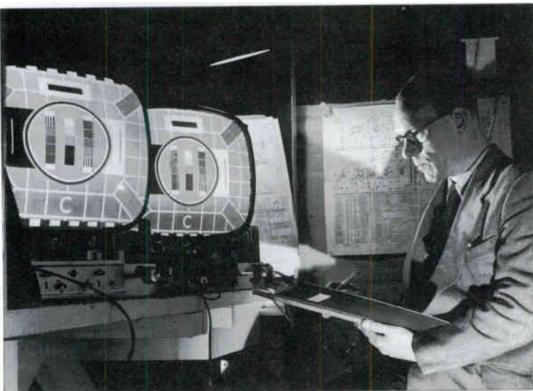
Quality control, c. 1960. Receivers taken from production lines are tested for consistency and reliability
