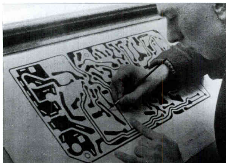
A draughtsman inking in the tracks on a printed circuit board at Ferguson in 1958. Note the wide spacing between tracks used in this early technique
