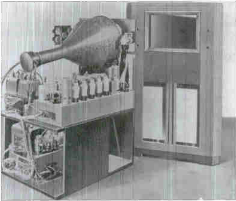
The GEC 12" receiver BT3701, showing its three massive chassis and the depth necessary to accommodate the electrostatically deflected tube
