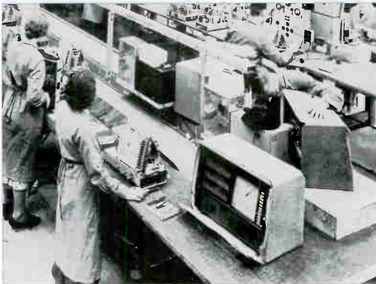
Ekco receivers of 1938, with motorized push-button tuning, undergoing initial wrapping before being boxed
