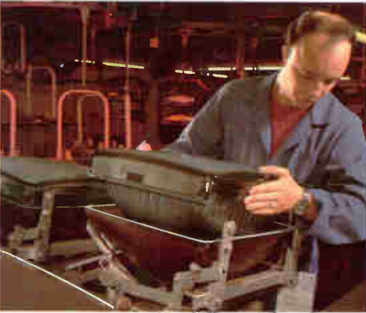
Placing the faceplate on the cone prior to fusing the two together, 1989. Care is needed in this operation to ensure that the spreading of 'frit' paste between the two is uniformly compressed
