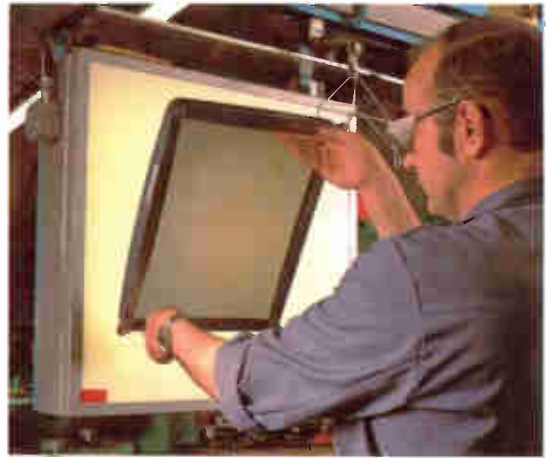
Examining shadow mask for defects, 1989
