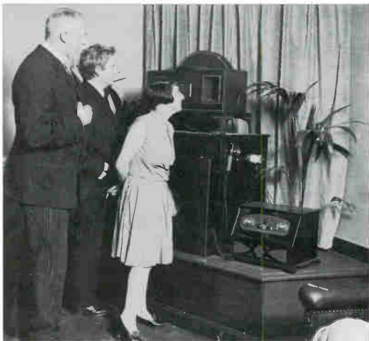
Baird demonstrates reception of 30-line pictures, transmitted by the BBC, at his Long Acre premises in about 1930. The Televisor is one of the 'production' models made by Plessey
