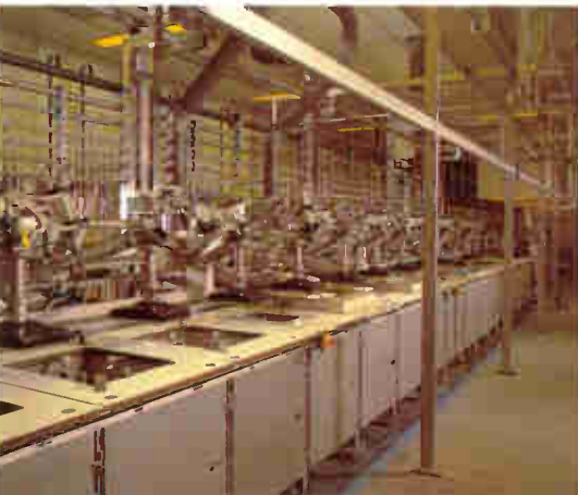
The automated production line for applying the black matrix
