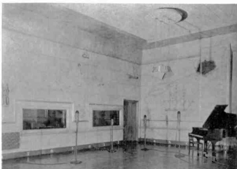
A CORNER OF THE "WORLD STUDIO" OF THE COLUMBIA BROADCASTING SYSTEM. NUMBERS AND LETTERS ON THE BASEBOARDS ARE USED BY INSTRUMENTALISTS TO MARK THEIR CORRECT LOCATIONS IN RELATION TO THE MICROPHONES.
