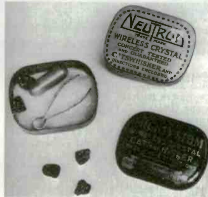
1920s Radio crystals complete with tweezers and instructions.
