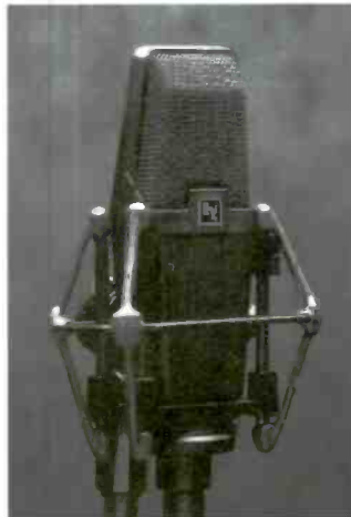
Electro-voice RE2000 with internal system to regulate temperature and humidity.
