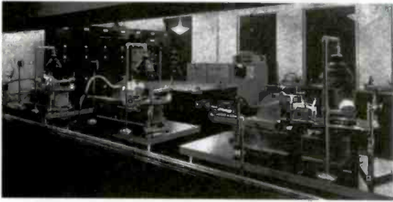
Cutting lathes for electrical transcriptions at NBC, 1940s.
