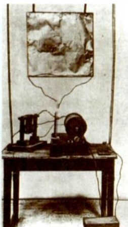
In 1895, Marconi achieved transmission of almost two miles using an antenna and ground at both the transmitter and receiver.
