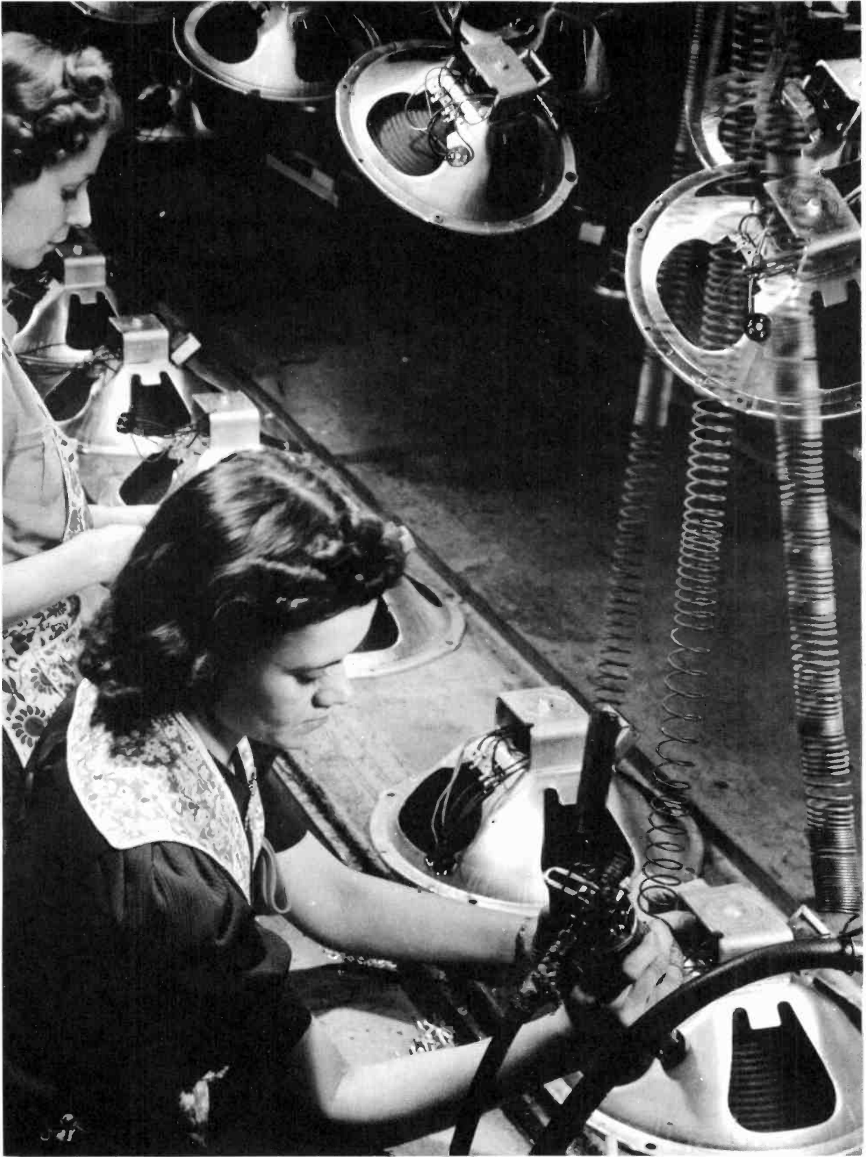
Assembling loud speakers. Part of the job of making your radio set.
