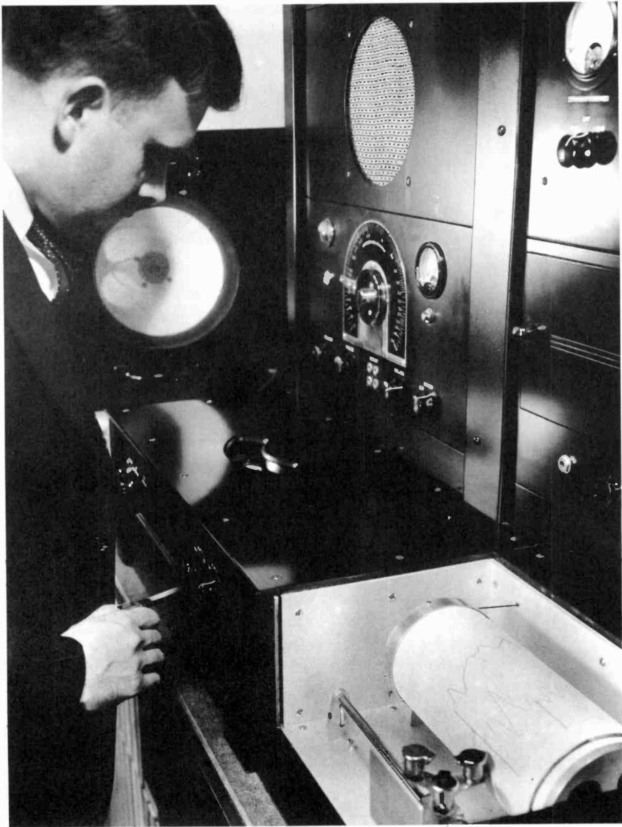
Loud-speaker response meter. Mr. R. Hackley operating semi-automatic device for checking response of loud-speaker. Charting roll in the lower right corner.
