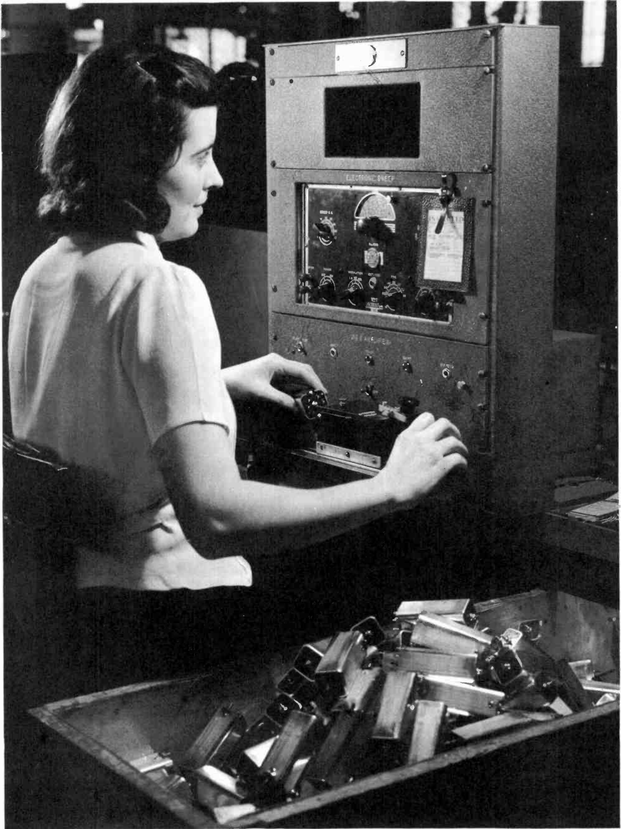
Transformer test. These transformers are used in superheterodyne receivers and accurate adjustment is necessary to provide proper operation.
