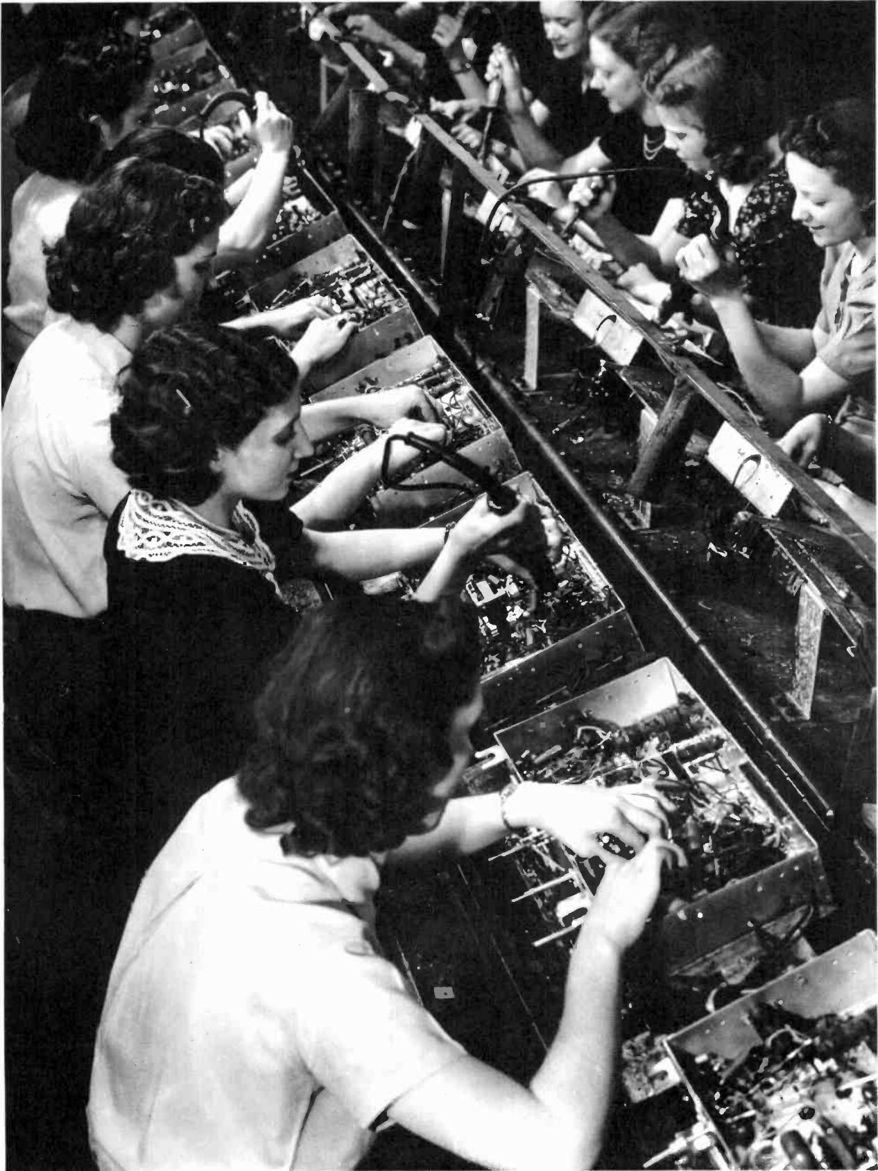
Radio receiver chassis assembly line. Girls soldering wires and small parts in position.
