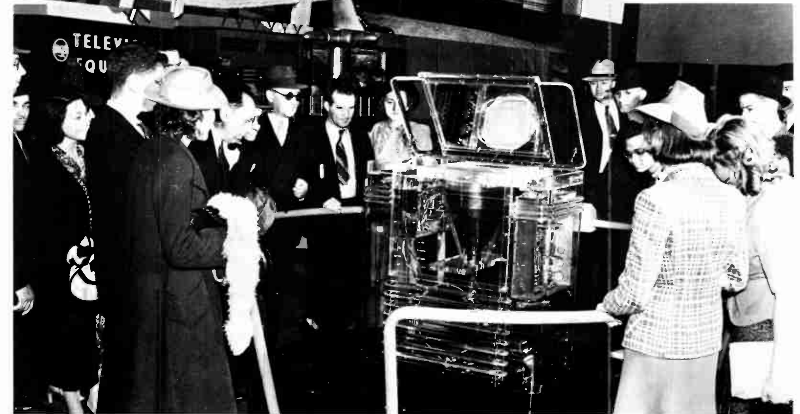
Above: A see-through television receiver with an 8 x 10-inch screen attracted a lot of attention at the 1939 New York World's Fair.
