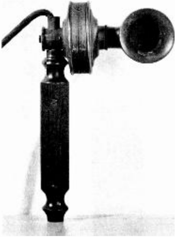
EARLY CARBON MICROPHONE Used with de Forest wireless telephone sets installed on vessels of the United States Navy during the world cruise of 1908.
