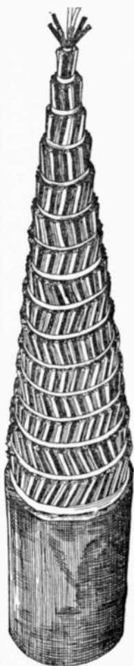
END OF TELEPHONE CABLE
