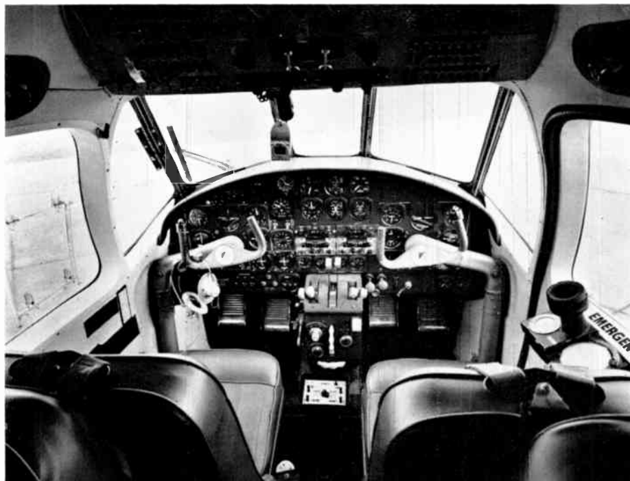
20. Flight panel of the Company's Piaggio 166 aircraft, used as a flying exhibition/test-bed
