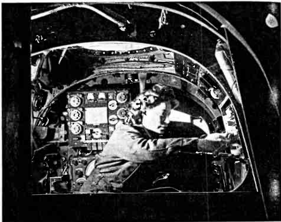
10. Routine maintenance in a wartime bomber aircraft. In the background can be seen the Marconi transmitter-receiver T1154/R1155, of which over 80,000 were manufactured
