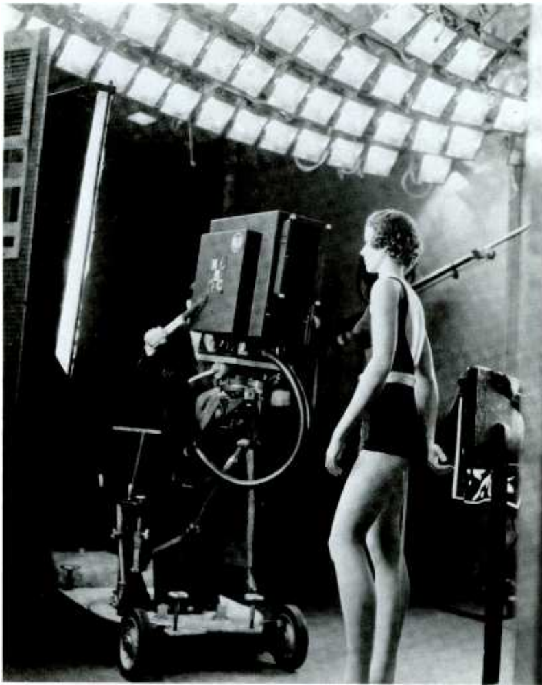
When NBC began experimenting with television from its 30 Rockefeller Plaza headquarters in 1935, they used this model, dubbed "Miss Patience," as a target for the testing of this first-generation iconoscopic camera.
