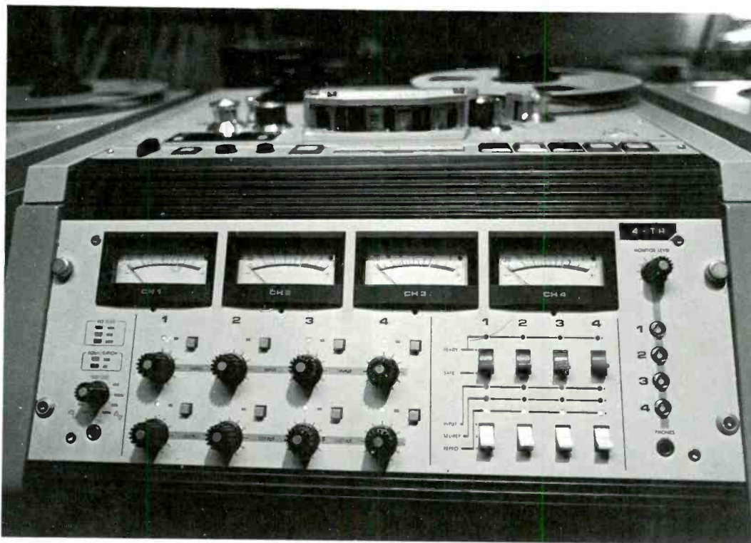
FIGURE 9.11 Four-track reel-to-reels are the most common multitrack recorders at radio stations. Courtesy WMJX-FM.
