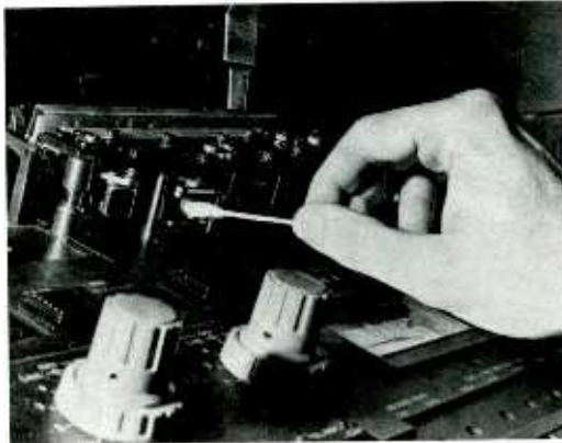
FIGURE 9.18 Dirty heads can create numerous problems, not the least of which is a deterioration in sound quality.
