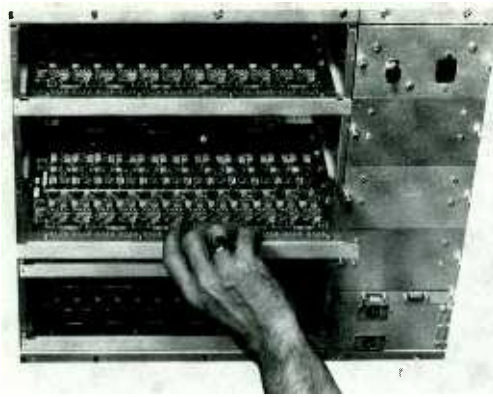
FIGURE 10.19 The luxury of solid-state electronics—pull out the bad, put in the good. Courtesy IGM.
