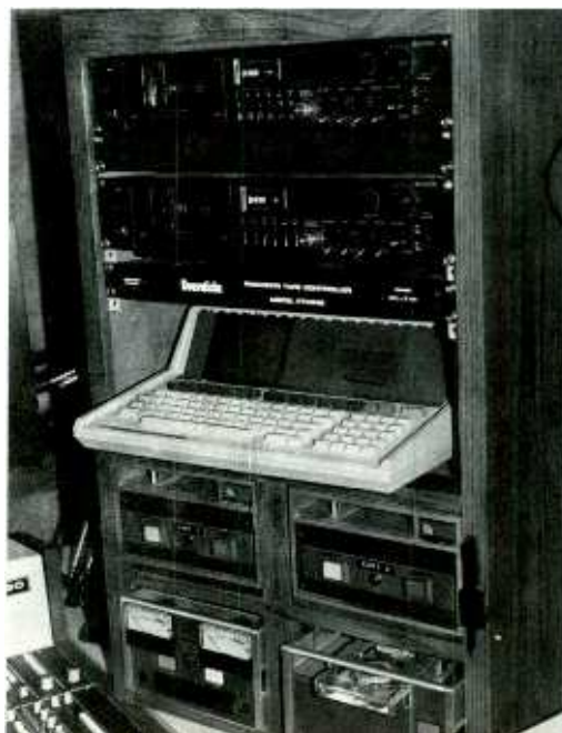
FIGURE 9.17 Equipment rack containing cassette tape machines, cartridge machines, and computer terminal. Rack mounted for convenience and ease of handling. Courtesy WMJX-FM.
