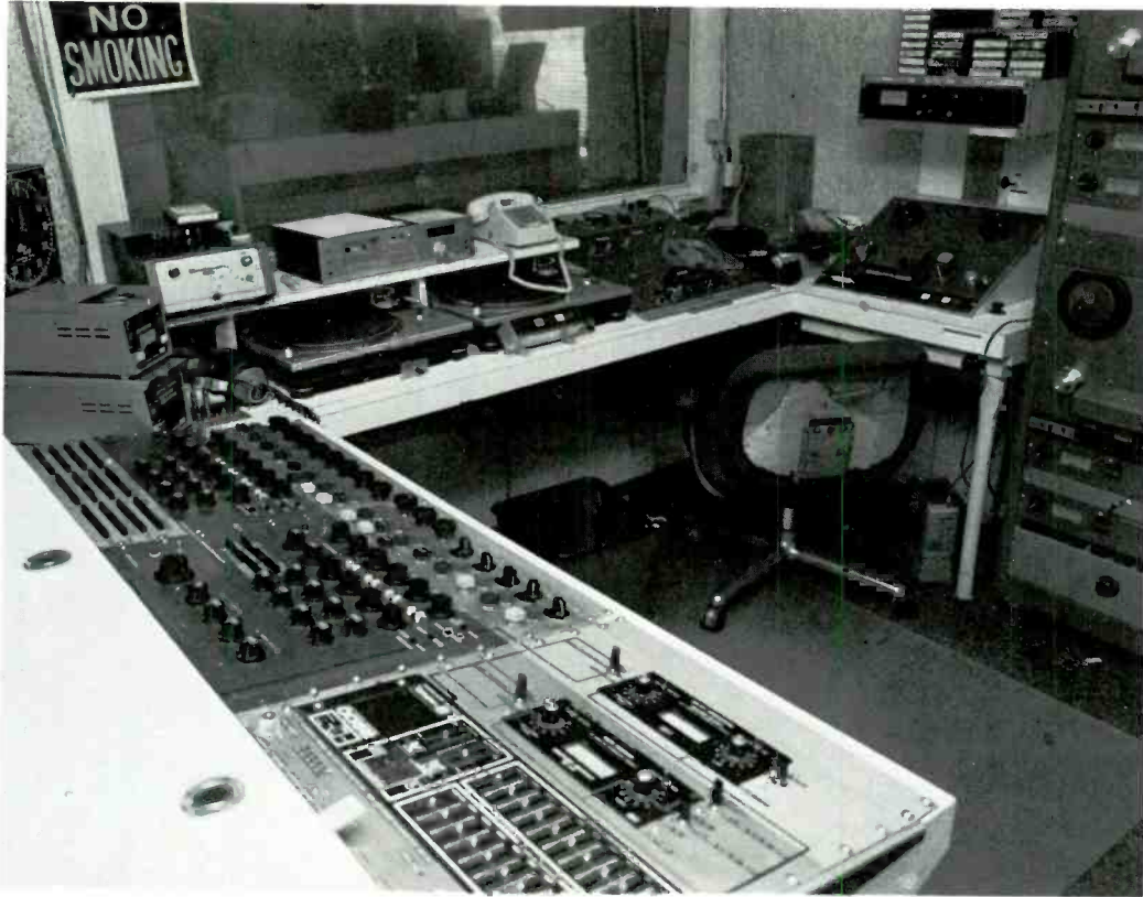
FIGURE 9.4 WHJJ/WHJY production studios. Although each studio is unique unto itself, the basics of layout are fairly consistent from station to station. For the sake of accessibility most studios are developed in a U shape, or a variation thereof.
