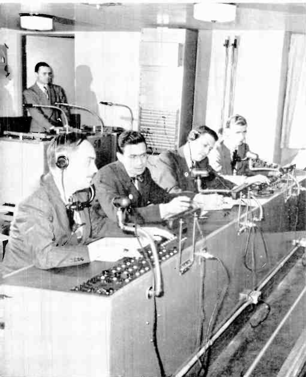
Scene in control room during production. Second from the left, front row, the director issues his orders to the technical director on his right and to the audio and video engineers on his left. His eyes are focused on the monitor, which is out of the picture. In the rear is the operator of phonograph turntables which supply appropriate music and sound effects.
