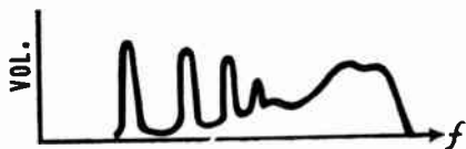
LINE AND BAND SPECTRA. Instantaneous content: here the sound is composed of individual tones superimposed on a broad spectrum band of noise.
