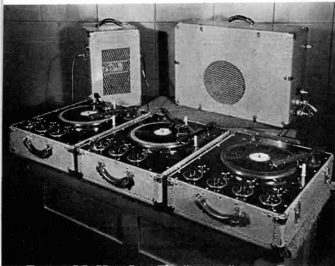
Figure 33. Turntables constructed as portable units.
