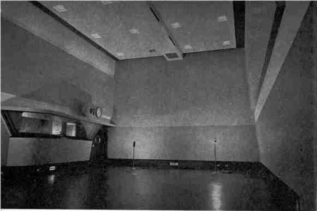
Figure 7. Live-end dead-end studio with slanting walls.
