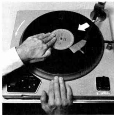
d. Backtrack the record. The turntable is in gear and all set to go.
