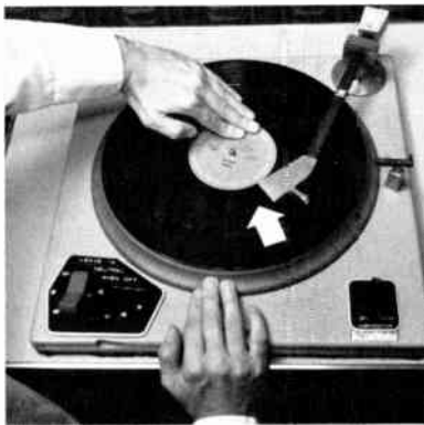
b. Spin the disc to find the first sound while holding the plate in place.
