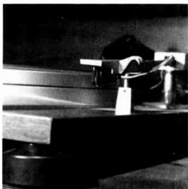
e. Cartridge and stylus.
