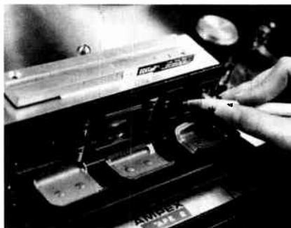
(b) Marking an edit point. Be careful not to get grease pencil on the head.
