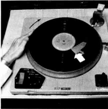
(a) The plate is spinning, but the disc is being held in place.
