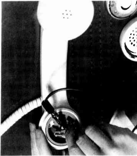
Figure 12.5 Tape recorder output cord with alligator clips, used to feed a recording directly into a telephone receiver. The reporter simply removes the mouthpiece and attaches the clips to the two prongs in the mouthpiece end of the receiver.
