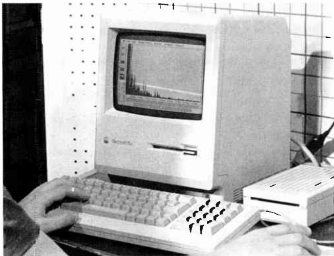
Figure 15.3 Sound envelope on a computer screen. This visual representation of sound can be easily and precisely edited.
