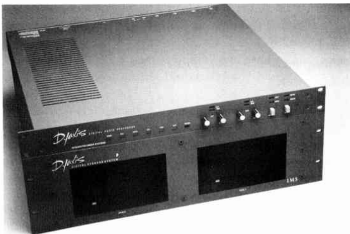
Figure 15.4 The Dyaxis Digital Audio Processor. This device makes it possible for a producer to assemble sound elements digitally, using a computer. (Photo courtesy of Integrated Media Systems, San Carlos, Calif.)
