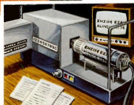
Outside broadcast units carry their own captioning machines (above), so that the scores can be superimposed on the picture.
