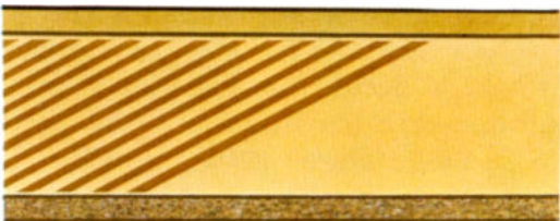
Below: Diagram of video-tape showing recording angle.
