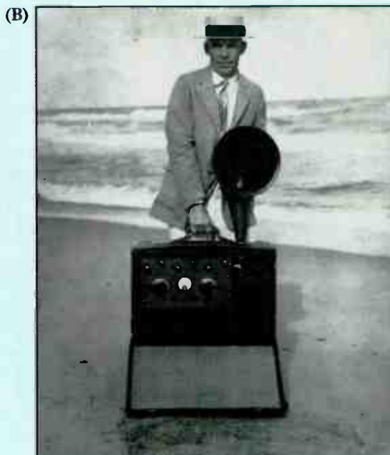
(A) The paper clip and pencil show the size of 1950s vacuum tubes in relation to 1960s transistors and current integrated-circuit chips. (B) Cumbersome vacuum-tube portable radios required either large batteries or household electric power. (C) Transistors began to replace vacuum tubes in the 1960s, leading to small, inexpensive portable radios. (D) In the late 1970s tiny portable television-receivers using integrated circuits became available.
