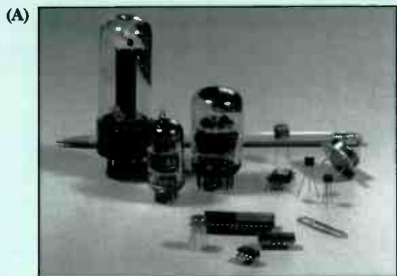
(A) The paper clip and pencil show the size of 1950s vacuum tubes in relation to 1960s transistors and current integrated-circuit chips. (B) Cumbersome vacuum-tube portable radios required either large batteries or household electric power. (C) Transistors began to replace vacuum tubes in the 1960s, leading to small, inexpensive portable radios. (D) In the late 1970s tiny portable television-receivers using integrated circuits became available.
