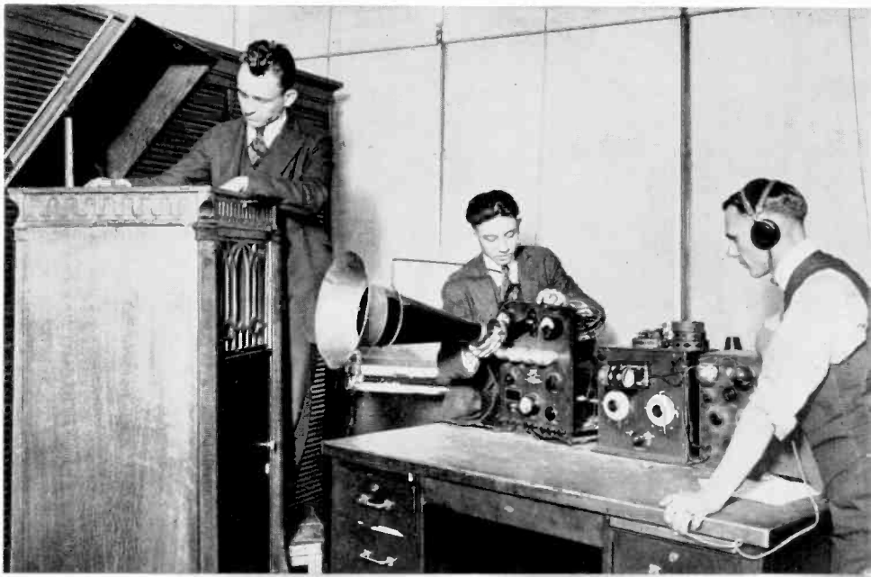
WWJ, Detroit, in 1920, showing crude method of acoustical pickup of phonograph records wwj
