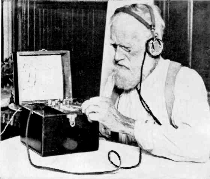
Typical crystal set of the earliest days of broadcasting (see p. 108) The Bettmann Archive
