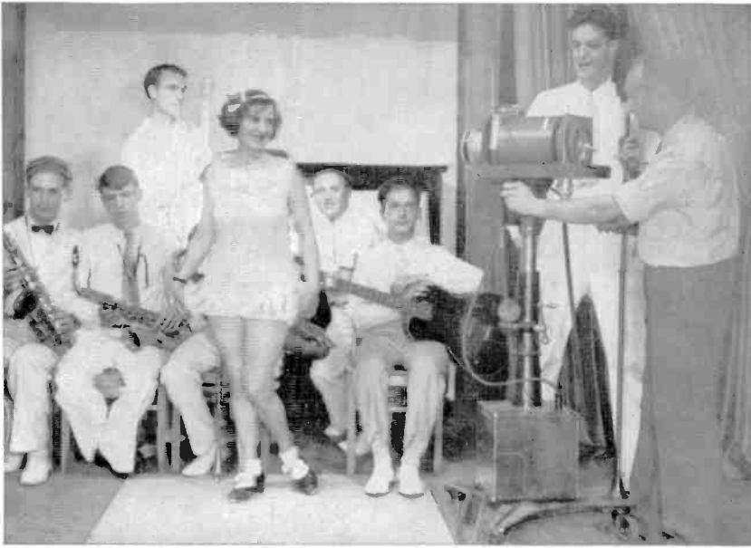
Farnsworth TV camera used in experimental productions in 1935 (see p. 155)
