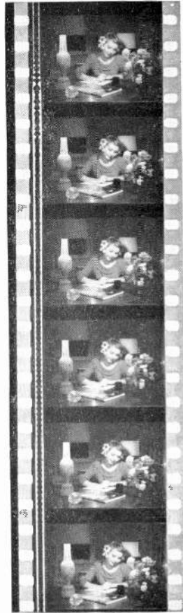
35-mm. variable-area optical track
