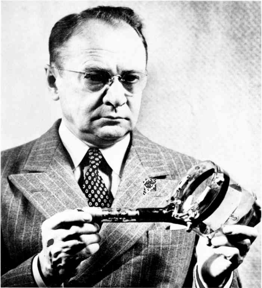
Vladimir Zworykin is holding a kinescope tube he used for picking up pictures and converting them into electrical images. As you can see, the tube is quite large, but it made possible the kind of television we enjoy today. (Culver Pictures.)
