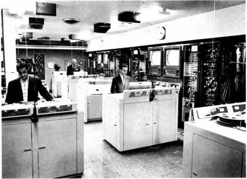
Fig. 8-1. Video tape recording equipment at NBC-TV's Tape Central in Color City Studios, Burbank, California. This operation is used primarily to record and play back shows to various legs of the NBC Television Network, thus eliminating the confusion previously caused in program scheduling by the semiannual shift to and from daylight saving time. (NBC-TV.)
