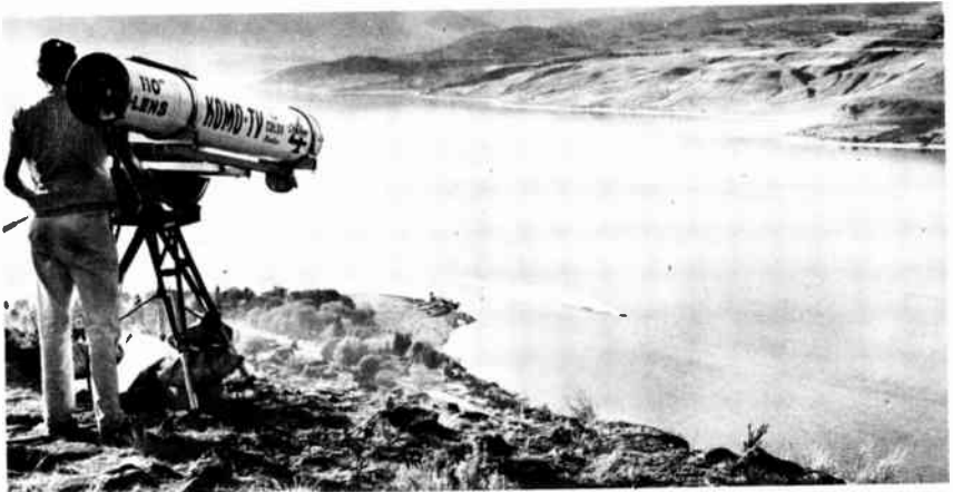
Fig. 5-3. An increasing number of television stations can originate live color television programs, and most stations can transmit network shows or film shows in color. Here a special 110-inch lens is attached to a KOMO-TV color camera to cover a hydroplane-racing special event. (KOMO-TV, Seattle.)
