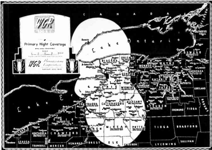
Fig. 11-1. Difference between daytime and nighttime AM radio station coverage. Radio Station WGR, Buffalo, uses a nondirectional antenna in the daytime (above) and a directional antenna in the nighttime (below). In general, the action of the Heaviside layer, reflecting the AM signal back to earth, extends the nighttime signal. In some cases, however, extended signals intermix, and the result is a decrease in nighttime coverage. (WGR, Buffalo.)
