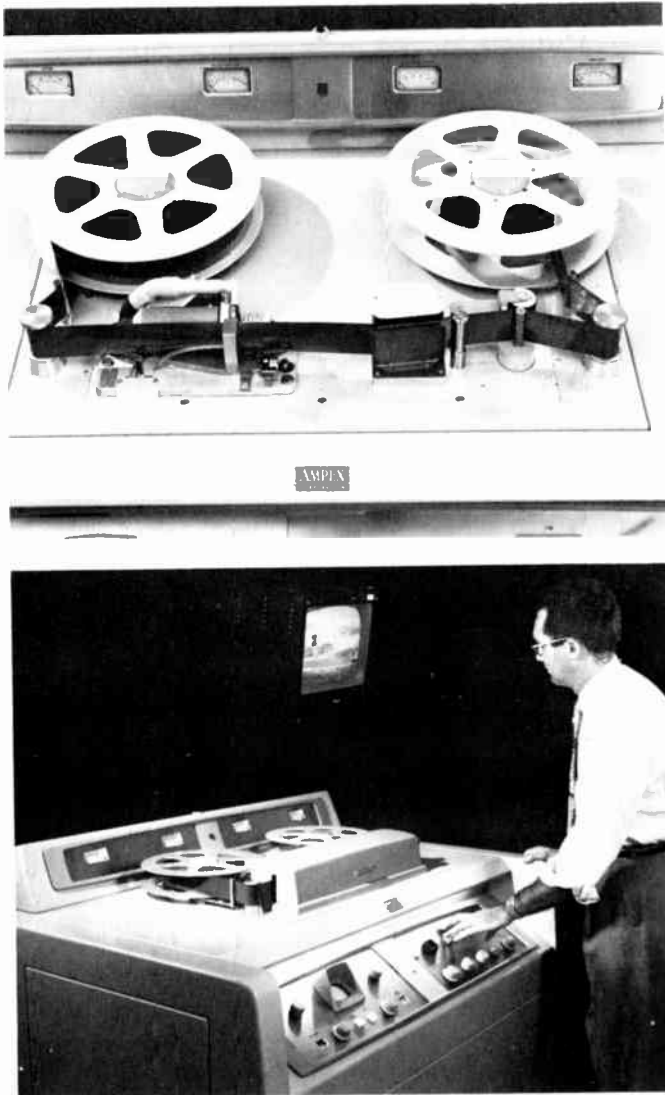
Fig. 8-4. Ampex VR-1000 video tape recorder. Above: A close-up of the tape moving through the heads with the protective cover removed. Below: The operator plays back a tape show, which can be seen on the monitor. By the addition of another bank of electronic equipment, the unit can be used for color as well as block-and-white operation. All Ampex machines have completely interchangeable units, and immediate playback is possible. (Ampex Corporation.)
