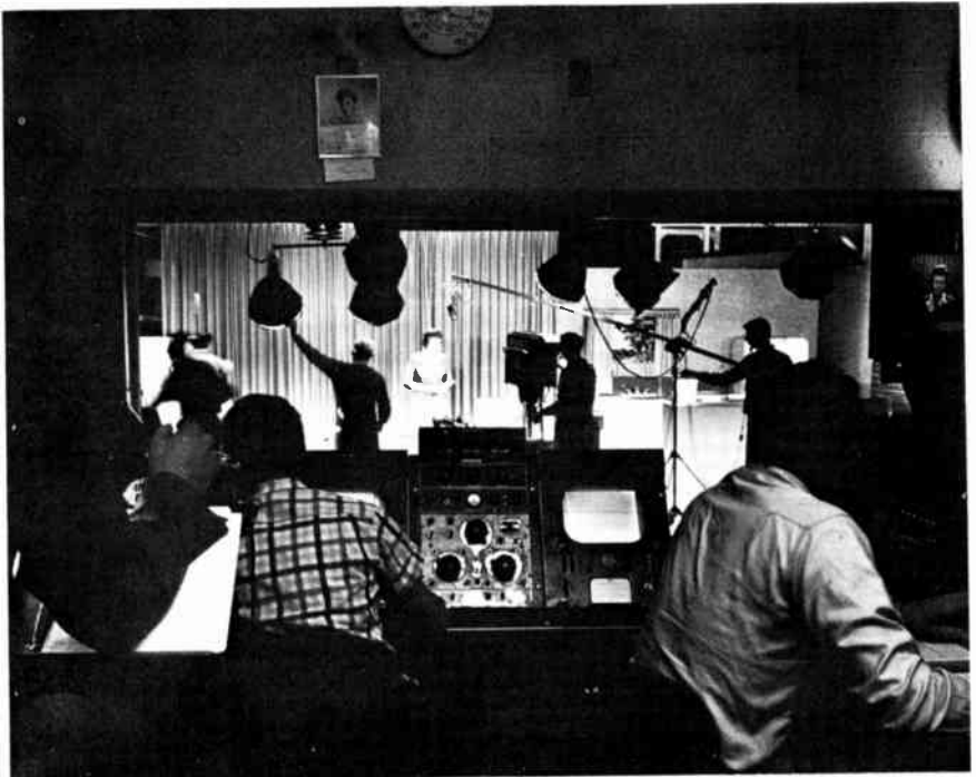
Fig. 2-2. A small-market television station on the air with a live show. WKOW-TV, channel 27, Madison, Wisconsin, surrounds its ABC-TV network schedule with numerous local community service programs, such as the homemakers' show seen through the control-room window. Left foreground: The director. Center: The video engineer. Right: The audio-transmitter engineer. Like most small-market station employees, WKOW-TV personnel double in brass in many assignments. (WKOW-TV, Madison.)
