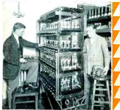
Over $100,000,000 worth of tubes are sold every year. This photograph shows two men testing tubes in a large manufacturing plant.
