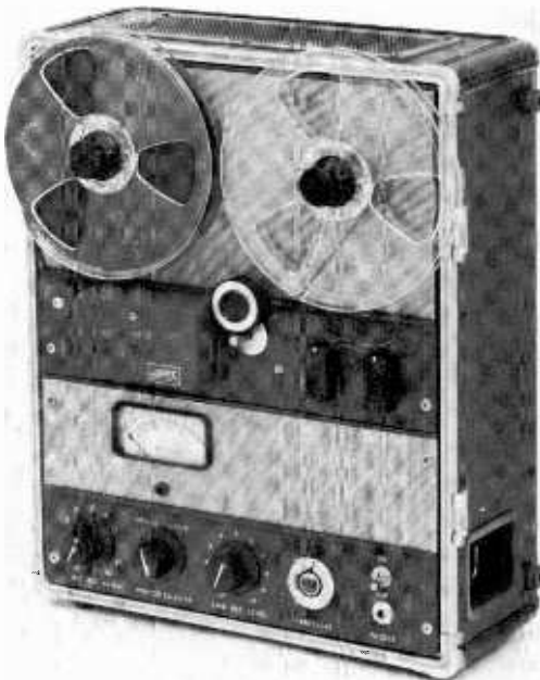
Fig. 6: Portable AC-operated broadcast-type tape recorder. Ampex 602.
