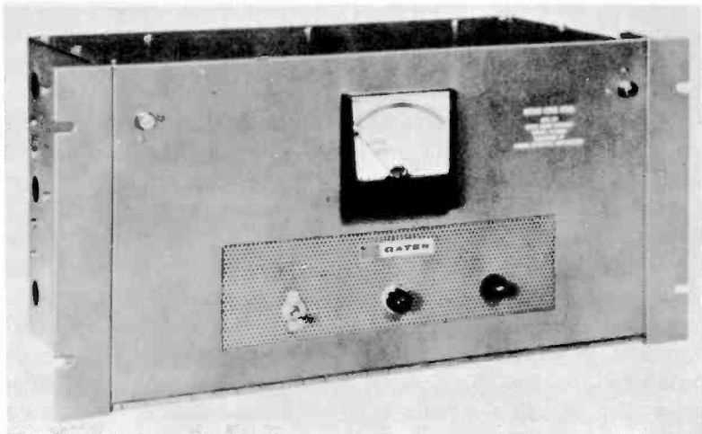
Fig. 7-13. A sophisticated automatic amplifier designed to distinguish between desired signal and noise levels (Photo courtesy of Gates Radio Co.).
