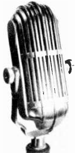
Fig. 16-7. An early unidirectional microphone incorporating two diaphragm dynamic generators, one of them modified for velocity response, stacked one above the other. A simple switch, not included, could have provided a choice of three patterns. With good directional properties, its inferior frequency and transient response made this public address unit unsuitable for broadcast purposes.
