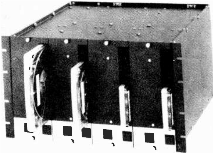
Fig. 8-7. Four independent cartridge tape mechanisms are combined in this modern single unit. (Courtesy of Sparta Electronics Corp.)
