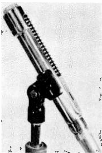
Fig. 16-8. A public address model with a frequency response entirely suitable for most remote applications, this Electro-Voice 676 obtains its unidirectional properties with a single diaphragm dynamic element and distributed rear ports acting through an acoustic network. Under $60.
