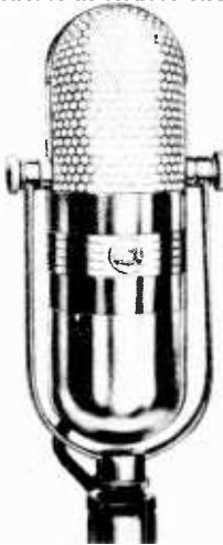
Fig. 16-6. An early and familiar multi-directional microphone using a single ribbon element and mechanically adjusted apertures to provide its various patterns. It, too, survives the years and is available today. (Courtesy of RCA)
