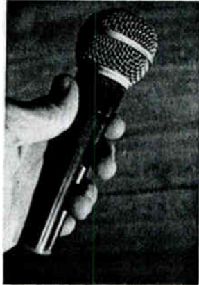
A microphone is a transducer that converts mechanical energy into electrical energy.
