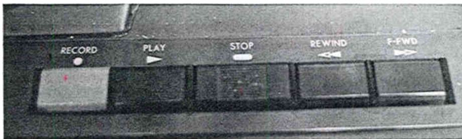
The transport controls on a popular open-reel machine include record, play, stop, rewind, and fast forward.
