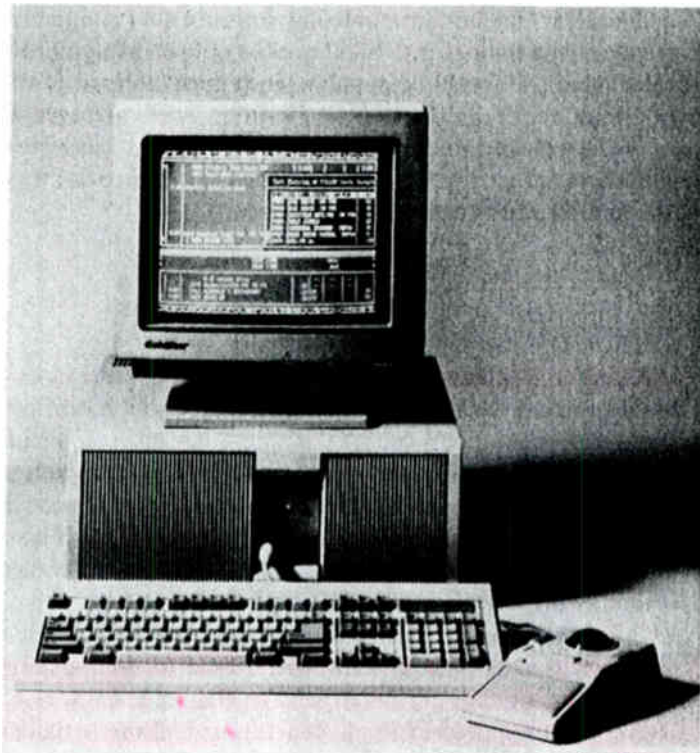
The Digital Commercial System (DCS) allows on-air playback of digitally stored commercials using a computer. (Courtesy of Computer Concepts Corporation)
