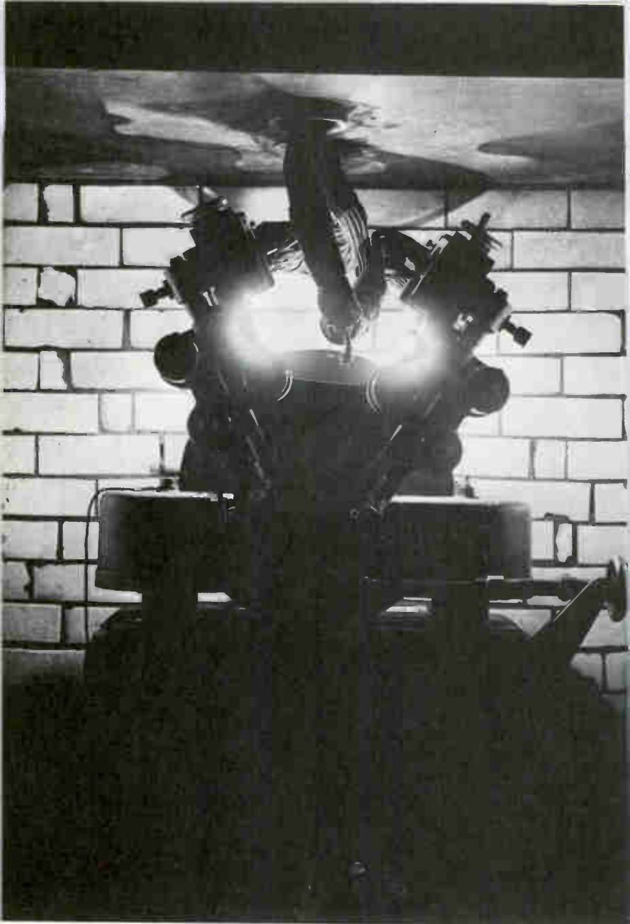
26 The huge synchronous disc spark transmitter set up at Poldhu in 1914. It is shown on the night of August 4th when it was transmitting the news of Britain's declaration of war on Germany to shipping. Soon after this these powerful spark transmitters were superseded by the far more effective diode, or radio tube.
