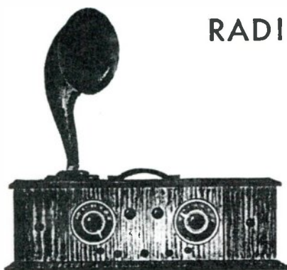
In the Mid-1920's, loudspeakers replaced earphones. Sets still used outside aerials (antennas).
