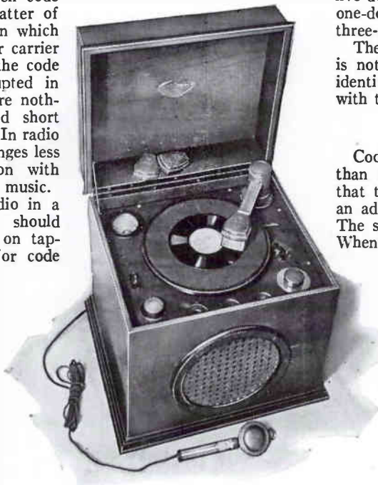
Above is shown a type of new home recording device which may be employed for making records of code transmissions which can then later be deciphered at leisure
