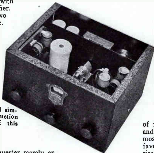
Figure 1. The fundamental circuit. The -24 and -35 tubes are, respectively, the detector and oscillator. The -26 tube is used as the power supply rectifier. The wave-change switch is not shown
