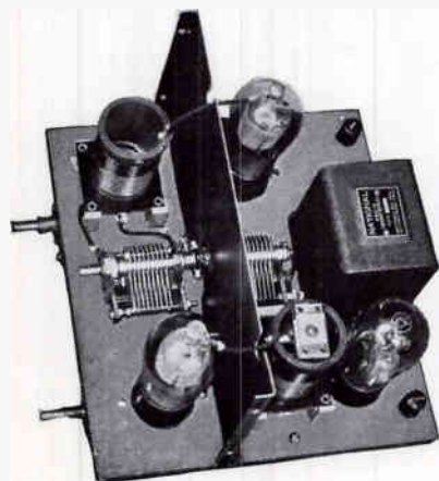
This looks like effective shielding, but as explained in the text it is not recommended for a receiver of this type. Scientific shielding is necessary
