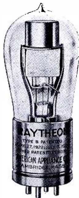
A closeup of the tube that acts as a check valve on the pulsations in the AC current of your light socket.
