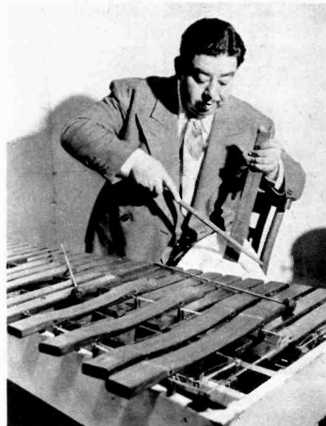
The marimba poses a real problem, must usually be sent back to the factory. Expert Jose Bethancourt shows how wooden keys are filed.
