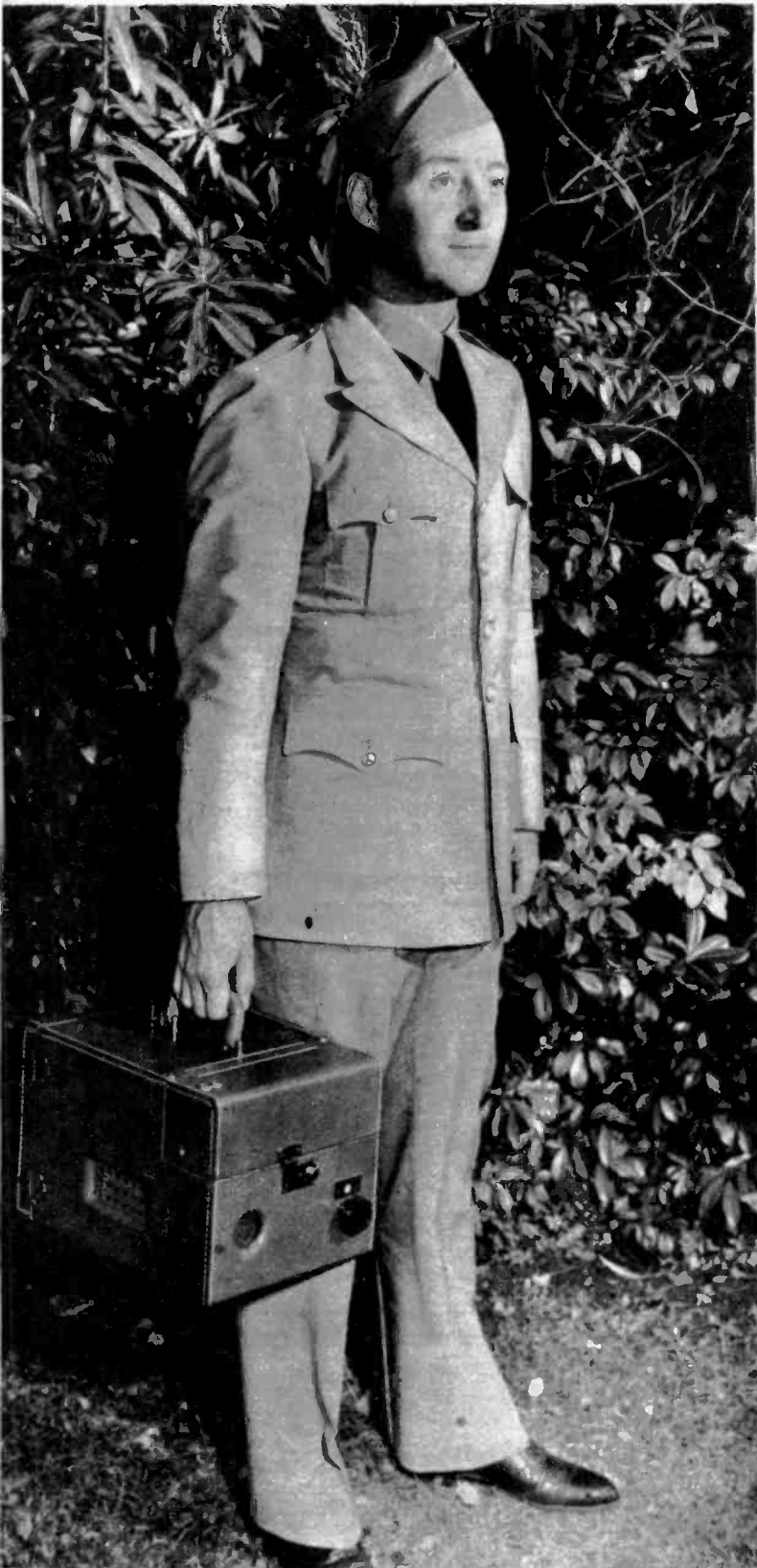
SOUNDSCRIBER IN HAND , Lawton is ready for action. The device weighs 24 pounds, records 30 minutes of conversation on a disc.
