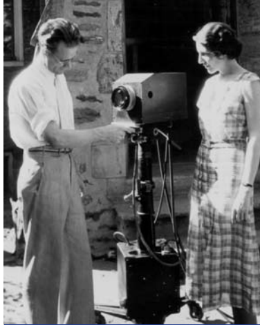
Philo T. Farnsworth and Mable Bernstein inspect one of the first portable TV cameras, built in 1934.
