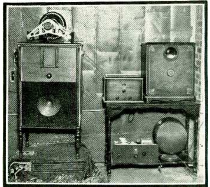
At the left in the above illustration is an experimental lens-disc projector constructed by the author. The disc and motor are sitting on the top of the cabinet. The screen is six inches square. At the right is a regular pinhole-type televisor.
