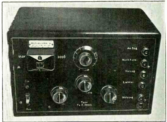
Fig. 4: Appearance of the neat and simple power-supply unit used with the latest Von Ardenne caenne cathode-ray receivers.
