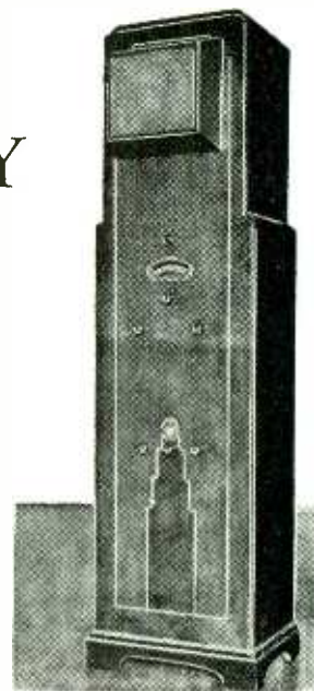
The mirror-disc receiver in its tall cabinet, which follows a popular design. The screen may be swung open to project a larger image.
