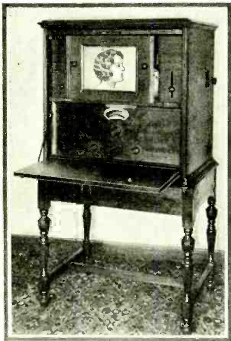
Fig. 3—Mr. Rosenthal's crater tube receiver, with his specially devised focusing controls.
