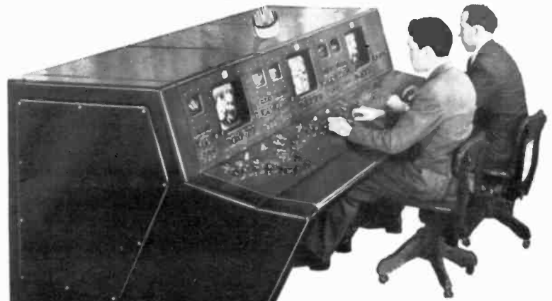
Du Mont Type TA-105-A Film Pickup Control Console. Includes saw-tooth, parabola and sine-wave shading with 5" waveform monitors for both line and frame. 12" picture monitor. Instantly accessible chassis. Integral design with the Du Mont Type TA-108-B Video Mixing Console and associated equipment which will handle four separate video or composite input channels with automatic or manual "fades" and "lap dissolves" between any video input channels.
