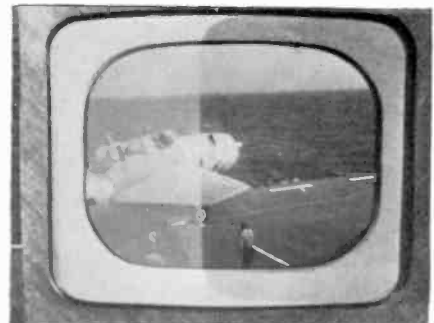
Here the advantages of a Polaroid filter are pointed up by this shot showing the "before and after" effect on the television screen.
