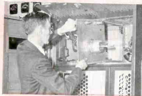
SIMPLIFIED TUBE CHANGING —When a PA tube change is necessary, the tube and special mounting plate can be removed as a unit and a spare assembly slid into place and connected in a matter of minutes.
