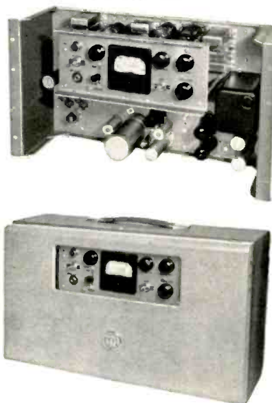
THE RELAY RECEIVER consists of the receiver unit itself, which is mounted on the rear of a parabolic reflector (and is similar in appearance to the transmitter unit) plus the receiver control unit shown above. The parabolic and receiver can be mounted on a permanent structure as shown at the top of this page or on a tripod similar to that used with the transmitter. The control unit is assembled on a bathtub-type chassis (top) which can be mounted on a standard rack or in a portable carrying case (bottom).
