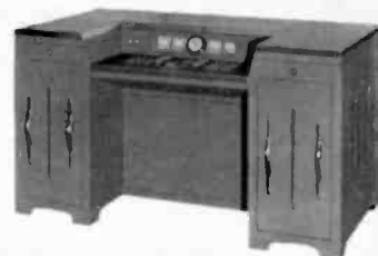
Farnsworth console for control of studio or film television programs, making possible the simultaneous operation of one or more television cameras.
