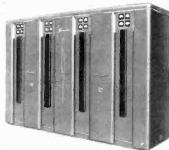
A four-kilowatt Farnsworth television picture transmitter.
