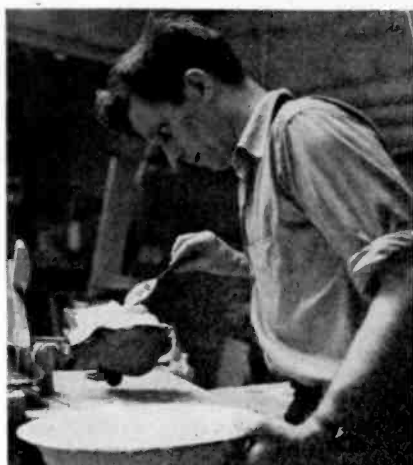
Plastic wood is then put into the cast of the model, and baked through a series of highly technical processes.
