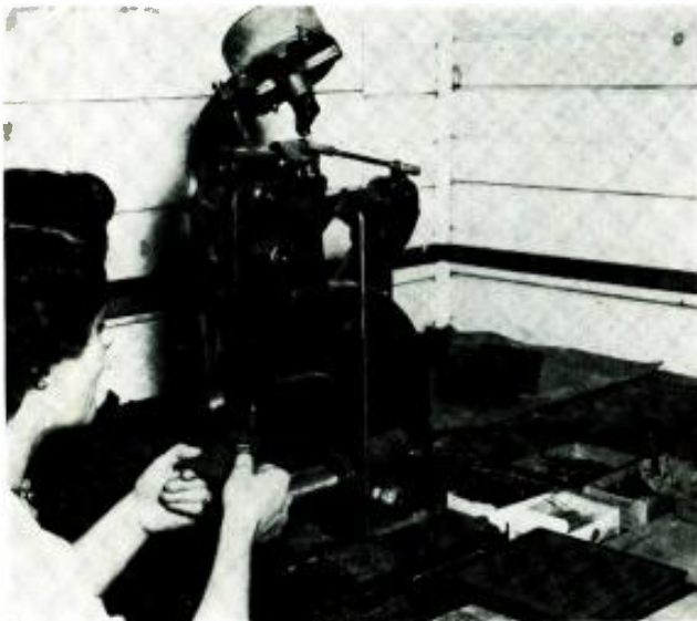
EYELETTING CIRCUIT pattern terminations for component lead insertions.
