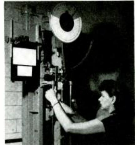
Determining tensile strength and ultimate elongation of polyethylene with special tester equipment (ASTM D-412-41) in the works control labs of the Bakelite Company.
