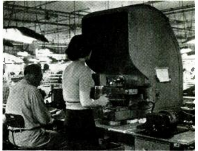
Optical comparator for control of winding machine setups.
