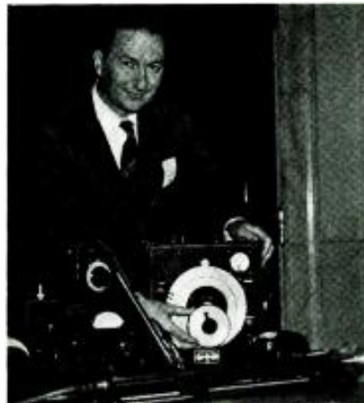
Frank Lewis, of General Radio, with a frequency meter designed for uhf work. At left appears an amplifier and null detector.
