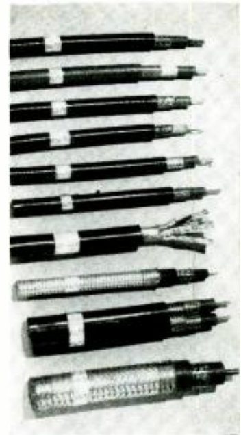
Assorted cables with polyethylene covers: RG 65/U used for spiral delay lines to provide a longer path for signal at high impedance; K-71 used in servo mechanisms; RG 9/U, a K456 silver-plated conductor and silver-plated braid used for uhf up to 3,000 mc in lead-in, test gear, probes, etc.; RG 11/U, a K-49 general purpose of shielded line; RG 63 A/U, a K-91 low capacitance rf cable used for test probes and applications requiring low capacity; RG 22/U, used as a balanced line for smaller df equipments such as those on planes and smaller naval vessels (also used successfully as FM and television lead wire); RG 8/U, a K-45 general purpose rf cable and transmission line, also used for special applications as power cable and high-voltage test probes; EX 610 cable, 5 par for pa systems; RG 12/U, K-49A general purpose rf cable armored for rough duty; RG 23/U, K602 power cable and highly balanced rf line for direction finder equipment (used in SCR-291 equipment during the war); RG 18/U, K12A heavy duty power rf cable used in df equipment and for shielded power lines, currently used in broadcast medium power antenna lead-ins and special train radio applications.
