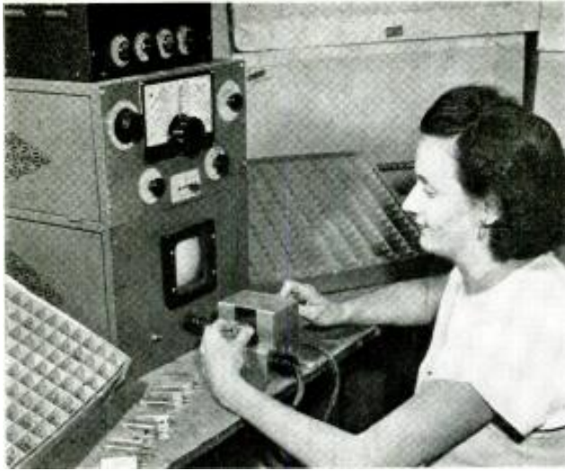
Final electrical test of if transformers.
