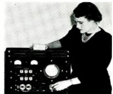
High-speed 'scope whose sweep speeds can be switched from 20 to 200 inches per microsecond. (Official USN photos)
