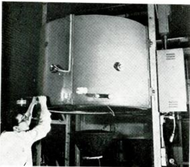
TV picture-tube baking and annealing oven located in G.E.'s plant at Syracuse. Oven, used for experimental work only, is located in the test lab of the tube building.
