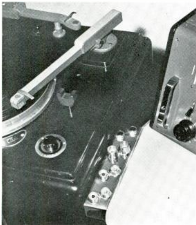
Chrome-plated shield cones used to protect remote-control tape buttons. From top to bottom: Pilot lamp to indicate when recording is being done; button to record; on button and last, off button.
