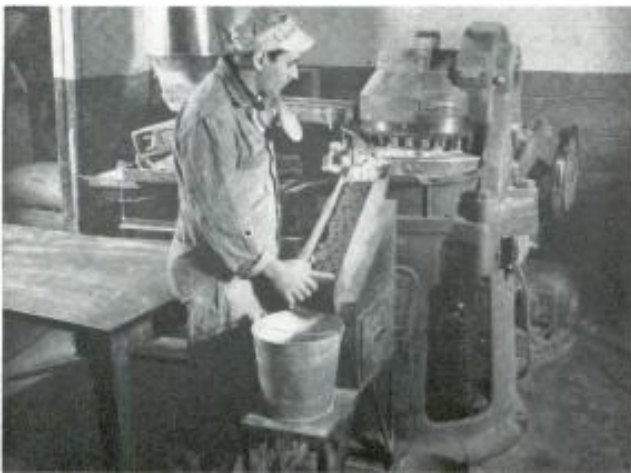
Pelleting glass-bonded mica 1, 2 for injection molding.
