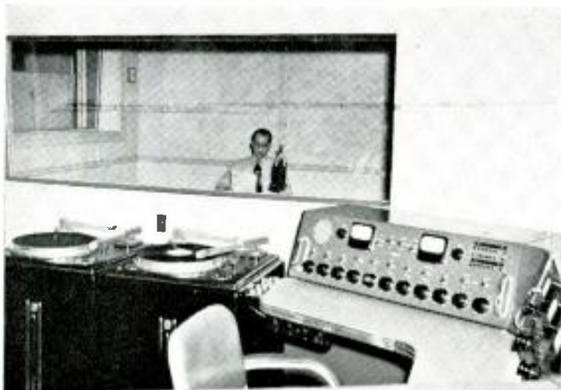
Section of master-control board that is directly related to the tape recorder operation. Buttons at top right control tape audio. Shield cones to right of right turntable contain remote push-buttons; see illustration on p. 28.
