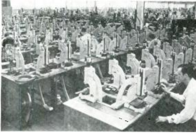
Kick presses employed in production of experimental fasteners. The experimental step involves the production of a design sketch, determination of the composition and gage of metal and equipment required, and the number of units to be made. This information is turned over to the development engineer, who, through consultation with the tool design superintendent, works out the design of tools necessary for production. The experimental part is then produced on a series of foot presses, with about 200 experimental pieces being produced, 50 going to the customer and 150 kept at the plant. The experimental setup is kept intact until the customer gives the part final approval.
