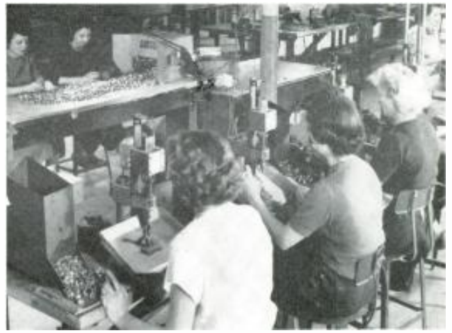
Socket center shield assembly and inspection.
