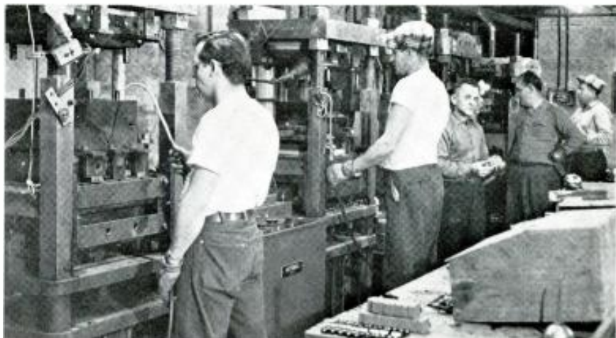
Above: Five 50-ton moulding presses being used for the manufacture of Vee-D-X lightning arresters and antenna insulators. Plant also has compression presses, ranging from 15 to 200 tons, for use with thermosetting plastics. A small injection press moulds small thermoplastic parts for use as insulators on antennas and for open transmission line. Left, top: Millen industrial version of its grid-dip meter. In addition to having an individually hand calibrated direct reading dial the model has an extended frequency range to cover the 220 kc to 300 mc bands. Left, bottom: RF capacitor, with a constant total capacitance and adjustable temperature coefficient, developed by NRL.
