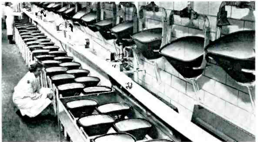
Quick drying method, in which tubes are placed in special drying racks (bottom of view). Process follows application of luminescent materials to the face plate of the tube.
