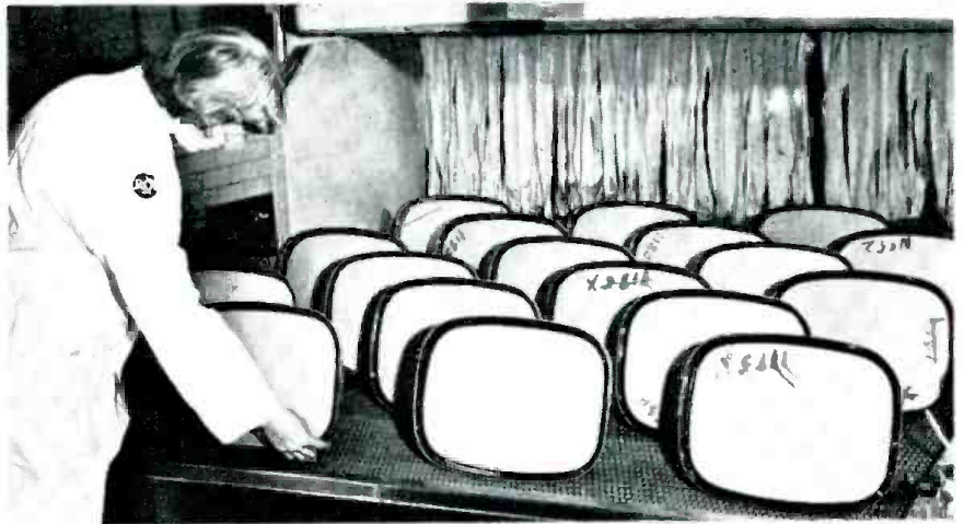
Glass-to-metal vacuum-tight sealing, at RCA tube department's Marion, Ind., plant. Glass face plate and the metal shell are placed on the rotating turntable of the machine where multiple oxygen fires form an oxide on the metal rim. The edge of the glass face plate is then melted in contact with the oxide-coated rim, to form the seal. A similar technique is used to bond the glass neck section of the tube to the smaller end of the metal shell.
