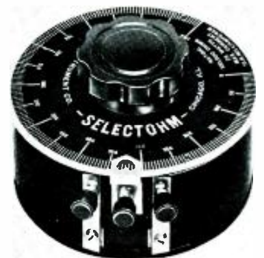
Left: Installing an adaptor plug from the decoder unit of a subscriber-vision picture unscrambler, into the sync socket of a TV chassis. Below: Calibrated 0 to 100,000-ohm linear potentiometer for use as a resistance substitute for service or laboratory work, which is said to provide a rapid means for determining the values of burned-out resistors when substituted in the circuits. (Courtesy Chicago Industrial Instrument Co.)
