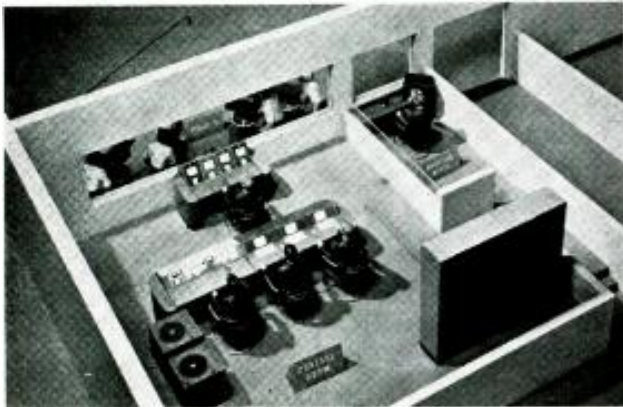
Figure 2 Audio and video console position, on a raised platform, behind the camera controls which may be adopted to permit program and technical directors to see their own monitors the camera monitors and also into the studio. Control room in front seats audio operator, program director and technical director. Announce booth is at left.
