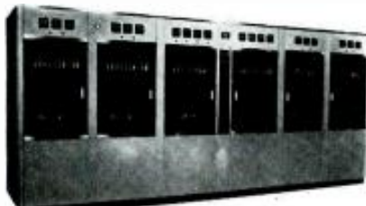
RCA 10-kw vhf transmitter
