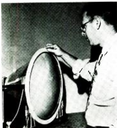
Left: Mounting a polyethylene plastic mounting ring on a 19-inch G.E. chassis to insulate the metal picture tube electrically. On the receding conical body of the tube is a sleeve of the same plastic, completing the insulation. The ring, patented by Anchor Plastics, was developed as a curved extrusion, a process designed to produce a curved shape free of distortion and of the tendency to straighten out again. It is claimed that circular, elliptical and other curved shapes for frames, mounts and the like can be extruded by this process to a maximum diameter of three feet. Right: Flexible electrical conduit, invented by Elliott Solero, of National Electric Products, which consists of an inner woven tubing made of longitudinal Fiberglas yarns, and a spiral wrapping of metal foil, with an outer braided jacket of aluminum wire. Conventional construction makes use of a spiral armor of interlocked aluminum strip over a braided aluminum wire jacket. Patent Office has granted patent number 2,514,905 on the conduit.
