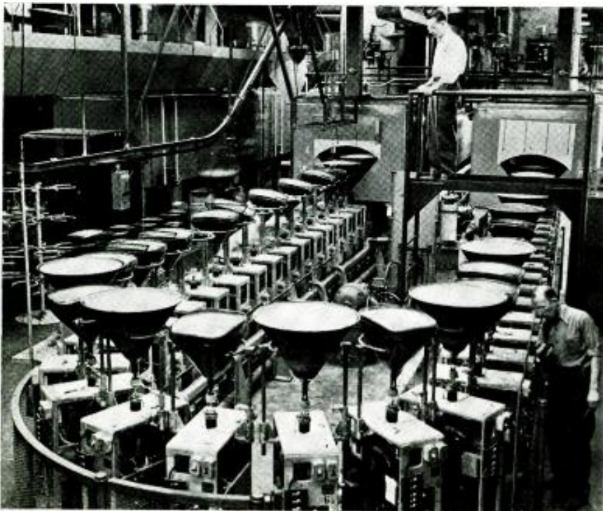
Left: In-line exhaust machine at the G. E. Electronics Park picture-tube plant which is capable of taking both round and rectangular tubes up to 24 inches in size. Each buggy has an oil diffusion pump which creates a vacuum. As the tubes move through a tunnel, they go through a bake-out process, which consists of heating each tube, to a temperature of 400°C, at which time the pump draws out the gases and other impurities. Below: Microwave-link antenna at Deer Island installation, used to transmit radar information from island to receiving station at Commonwealth Pier, South Boston, which served as a harbor radar centre for a recent test and demonstration by Raytheon and Port of Boston Authority.
