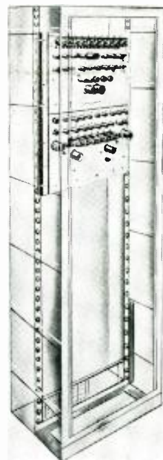
Synchronizing generator mounted in rack for studio application. Generator is constructed on two separate chassis, each 14" in height and designed to fit a standard 19" rack. Entire generator (both units), with all tubes and components, weighs 23 pounds. Each unit contains 27 tubes; a total of 54 tubes in the entire system. The circuits necessary for the establishments of the timing relationships are located on one chassis; the timer unit. The circuits necessary for the formation of the synchronizing signal and driving pulses are located on the other chassis; the shaper unit. Below: Generator in portable carrying case. The binary counters used in the main count down, (525-to-1) and in the synchronizing signal formation chain are of the individual plug-in type. Ten of these units may be seen in the recessed sub-assembly, the top of the timer unit. Each binary counter circuit is contained in a sealed unit which plugs into an octal socket.
